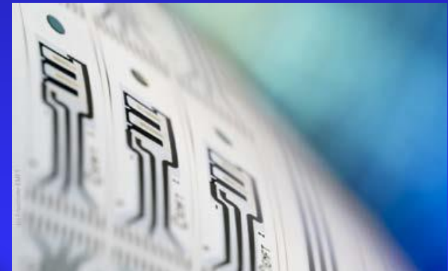
Printed conductive patterns used to create flexible Printed Circuit Boards (Source: ISORG)
